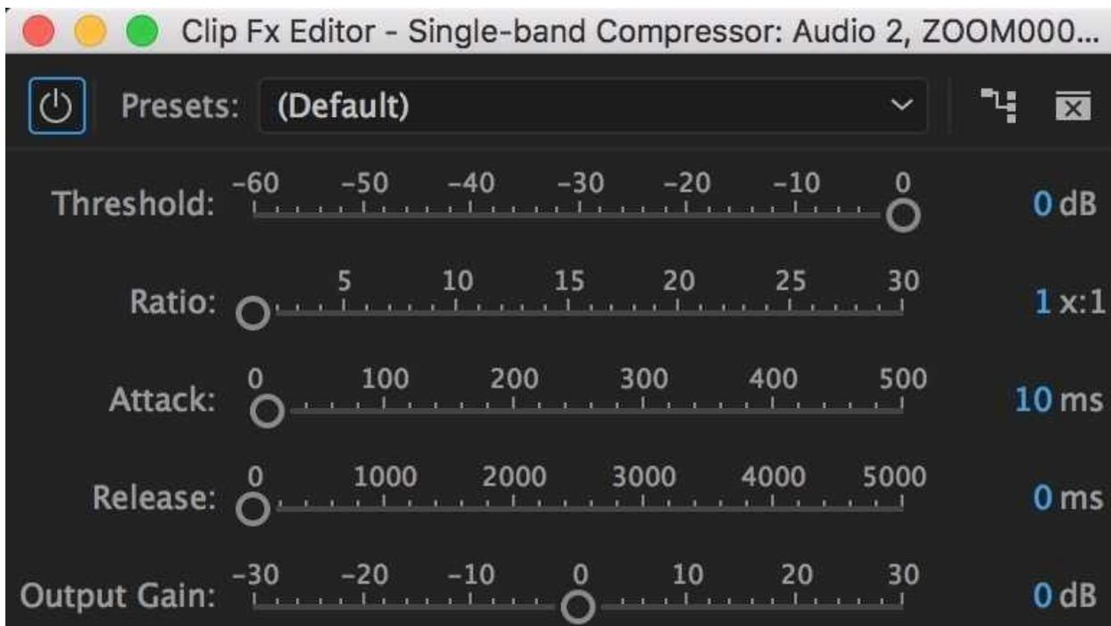
Compression reduces the dynamic range of audio, constraining the difference between soft and loud sounds in the mix.
