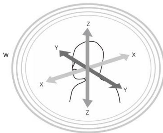
4 - With ambisonic recording on the H3 panning can be done around X, Y and Z planes.
