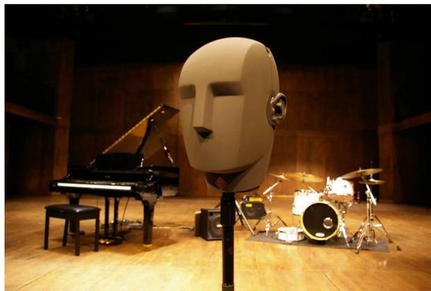
*2 - Headphones in the 'ears' of a dummy head can be used for binaural recording*
